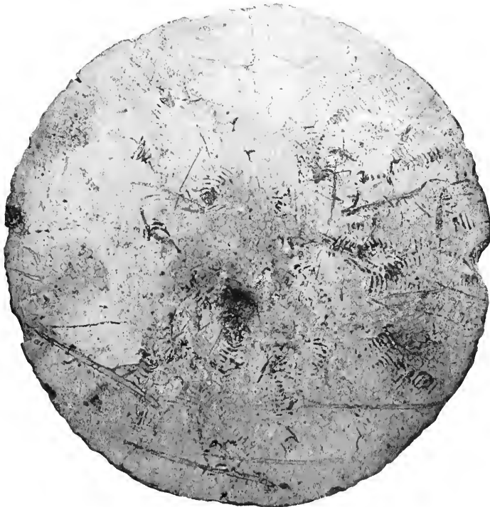
Pat made of Portland cement containing 6.23 per cent. of Alumina. Photograph taken when pat had been in concentrated sea water 77 days. First crack appeared on the 59th day.
